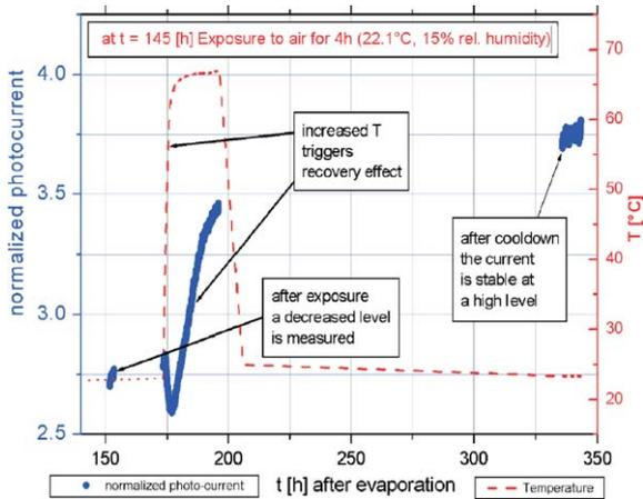
Fig. 5. Time development of  $\langle I_{\text{norm}} \rangle$  and  $T$  after exposure to humid air (extension of Fig. 4).
