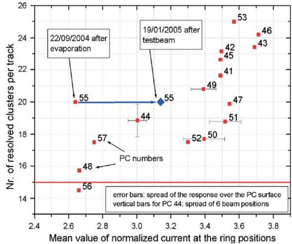
Fig. 3.  $N_{\text{CL}}$  in the beam plotted against  $\langle I_{\text{norm}} \rangle$  at the position of the Cherenkov ring.
