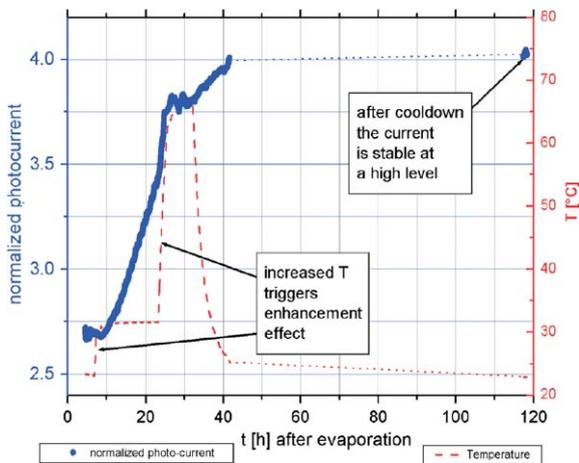
Fig. 4. Time development of  $\langle I_{\text{norm}} \rangle$  and  $T$  during heat enhancement phase.
