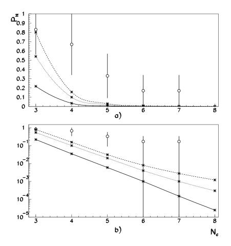
The alignment degree  $P_{N_c}$  as a function of cluster number  $N_c$  at h=50 m and  $\sqrt{s}=14$  TeV in linear (a) and logarithmic (b) scales. The solid curve is the result (coincident with one at h=1000 m)without restriction on the total cluster energy  $E_{\Sigma}^{\rm thr}$ , the dotted curve — at  $E_{\Sigma}^{\rm thr}=2$  PeV the dashed curve — at  $E_{\Sigma}^{\rm thr}=10$  PeV. Points ( $\circ$ ) with errors are experimental data.
