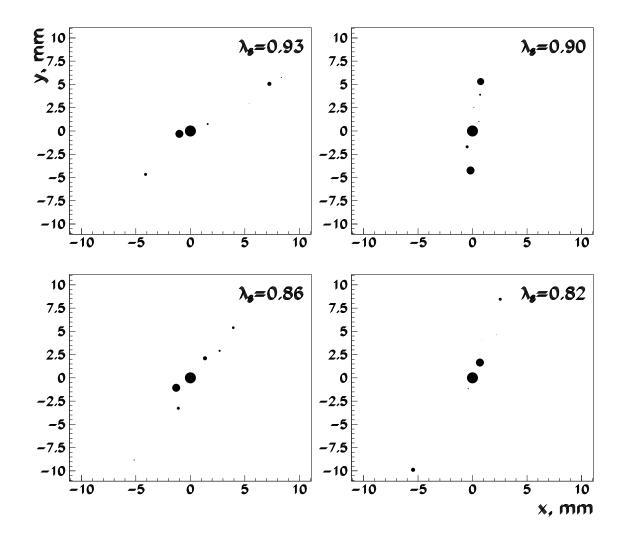
Samples of core distributions for simulated events with  $E_{\Sigma}^{\text{thr}} = 10 \text{ PeV}$  and  $\lambda_8 > 0.8$ . The size of spots is proportional to their energy (except for the central spot which is not to scale).
