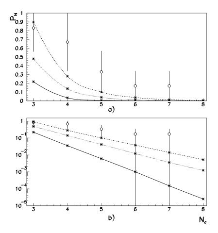
The alignment degree  $P_{N_c}$  as a function of cluster number  $N_c$  at h=50 m and  $\sqrt{s}=14$  TeV in linear (a) and logarithmic (b) scales. The solid curve is the result (coincident with one at h=1000 m)without restriction on the minimum value of process hardness  $p_T^{\rm hard}$ , the dotted curve — at  $p_T^{\rm hard}=300$  GeV, the dashed curve — at  $p_T^{\rm hard}=3$  TeV. Points ( $\circ$ ) with errors are experimental data.
